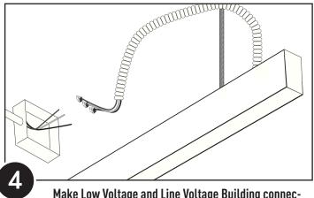
Make Low Voltage and Line Voltage Building connections with pre-attached flex conduit
