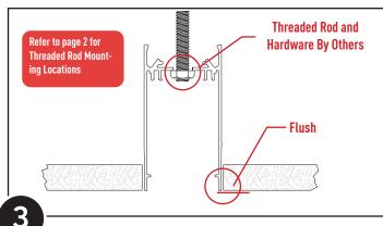
Connect Fixture to Structure with threaded rod (by others) and make sure bottom of fixture is level with ceiling surface
