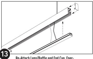
Re-Attach Lens/Baffle and End Cap, Energize Luminaire, You are Done, Great Job!!
