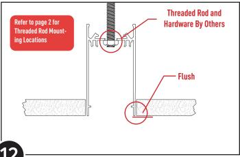
Connect Fixture to Structure with threaded rod (by others) and make sure bottom of fixture is level with ceiling surface
