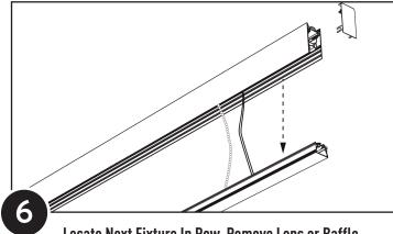
Locate Next Fixture In Row, Remove Lens or Baffle Assembly with Small Flathead Screw Driver or Pick
