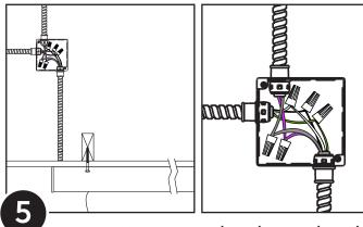
Make Wire Connections, Hot (Black), Neutral (White), and Ground (Green) connections, as well as Low Voltage Control Wire Connections (Purple, Gray)
