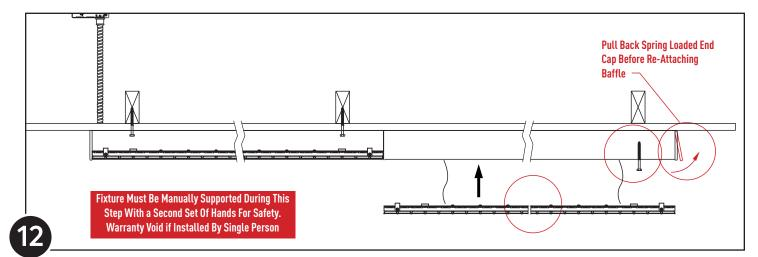
Secure Next Fixture Section To Structure (only one mount necessary) with Appropriate Hardware (By Others) and Snap Baffle Back Into Place
