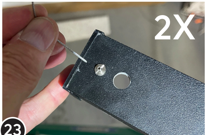
Insert Aircraft Cable Into Cable Fitting on the Power and Non-Power End of Fixture
