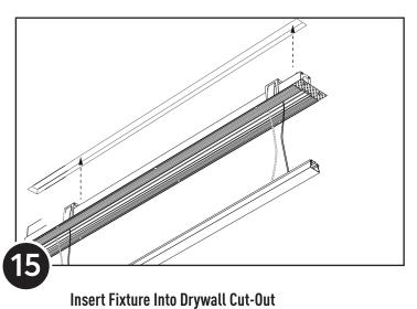
Fixture Must Be Manually Supported During This Step With a Second Set Of Hands For Safety.
