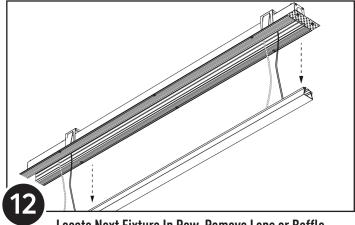
Locate Next Fixture In Row, Remove Lens or Baffle Assembly with Small Flathead Screw Driver or Pick
