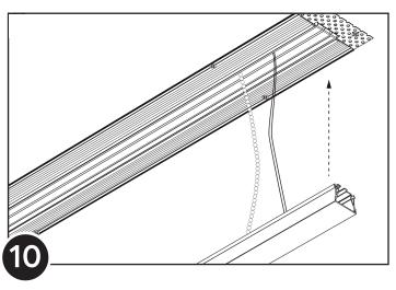
**Snap Lens or Baffle Back Into Fixture Aperture**
