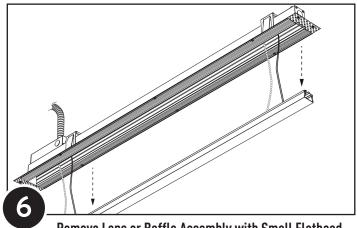
Remove Lens or Baffle Assembly with Small Flathead **Screw Driver or Pick**
