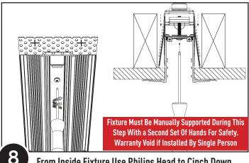
From Inside Fixture Use Philips Head to Cinch Down Yoke Bracket By Rotating Screw Clockwise
