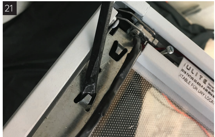
You may have to slightly bend tabs upward with a flat head screw driver to allow for full engagement
