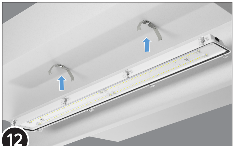
Snap fixture into place, ensuring brackets overlap the fiberglass body
