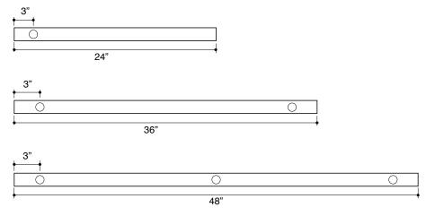
Nominal 6' and 8' are made up of joining two nominal 3' or 4' housings together.
